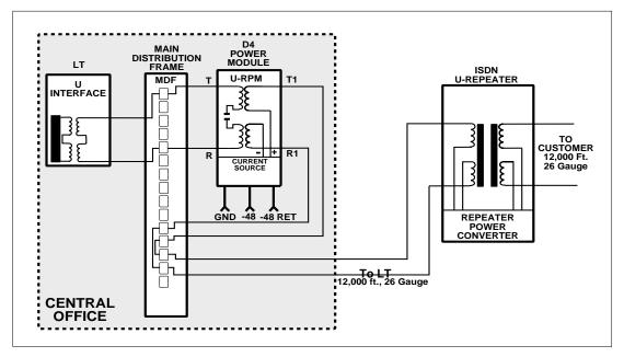
FIGURE 2. U-Repeater Powering Module Application
